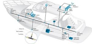
Watercraft can avoid the need for large instrument clusters and multiple displays and readouts by connecting systems as diverse as tachometers, fuel & oil sensors, satellite radios, and wind transducers to the marine panel pc. Via a networking protocol called NMEA 2000 or NMEA 0183, watercraft electronics can communicate with each other seamlessly, and a single display panel can provide all of the needed
