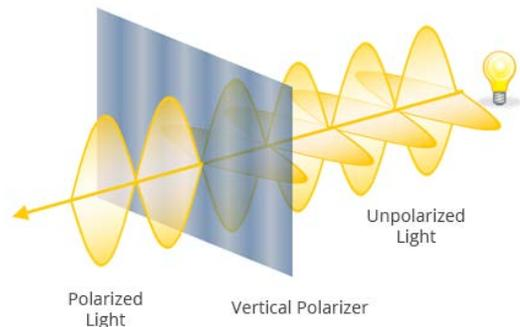
Basically, a polarized lens blocks out light coming in at angles and brightness levels that are consistent with reflections, while allowing light that is consistent with normal sources to pass through.<sup>3</sup> Unfortunately, under some circumstances, this type of film may block out light from a tablet screen, causing it to appear black. This can usually be fixed by turning the tablet to a different orientation, but often that's not really a reasonable solution.
